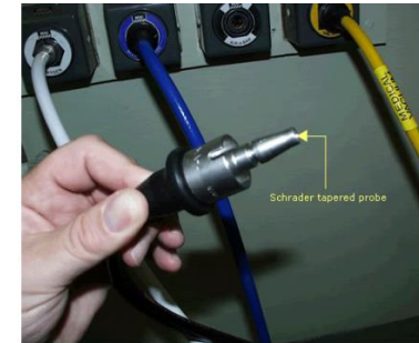
Fig 1 Schrader tapered probe
