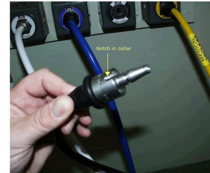
Fig 4 Notch in collar
