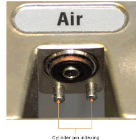
Fig 1 The yoke side of the system
