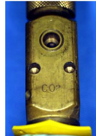
Fig 2 Holes in cylinder which match pins in the yoke
