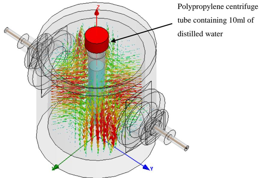
Figure 8: TE<sub>211</sub> mode for large volume cavity, simulated with a water sample at the centre.
